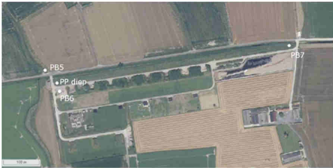
Figure 3.4: Four new wells installed by De Watergroep in June 2024 (PPd is an extraction well for brackish groundwater; PB5-7 are monitoring wells).
