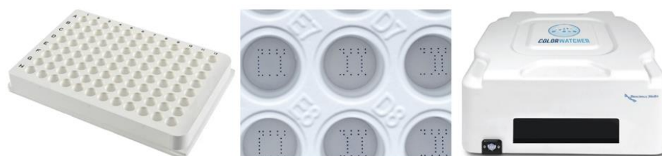
Figure 13. Microtiter plate (left), a microarray of spots in wells (middle), and an automated microtiter plate image reader from Bioscience Media that returns results in five minutes (right).
